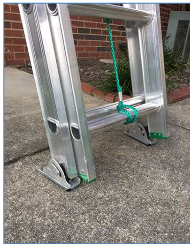
Figure 3. Ladder feet resting on cement
