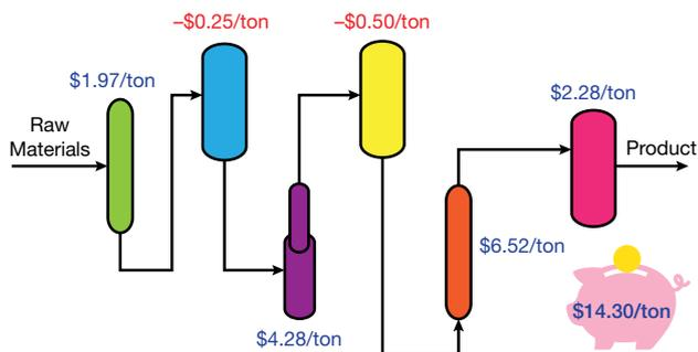
▲ **Figure 5.** The production control layer coordinates multiple APCs to control the entire plant as a single entity. Optimum operation of a single unit does not necessarily benefit the entire process. It may be better to run some units below their optimum point to obtain a larger overall benefit.
