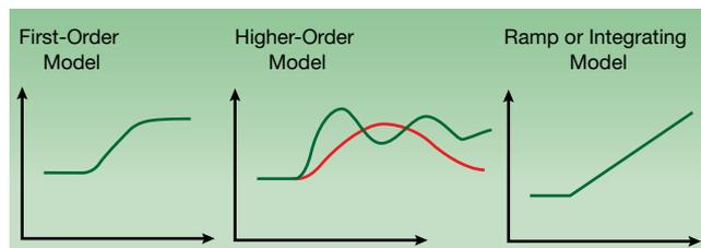
▲ **Figure 3.** First-order models have a simple and predictable response, whereas second- and higher-order models can have multiple peaks and valleys. Ramp or integrating models imitate the level of a tank: if the input and output flows are equal, the tank level remains constant, but if there is a disparity, the tank will overflow or empty.
