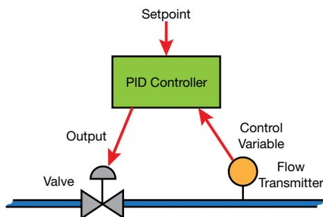
▲ **Figure 2.** The PID control block compares the user-specified setpoint (SP) to the control variable (CV) measured by instrumentation, such as a flow transmitter, and provides an output (OP) that manipulates the process, such as opening or closing a valve.
