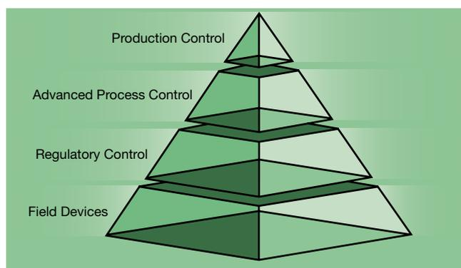
▲ **Figure 1.** Process control consists of four tiers: field devices, regulatory control, advanced process control (APC), and production control.
