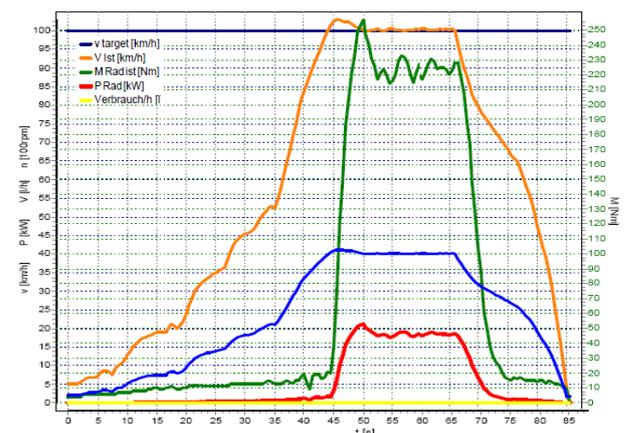
Fig. 4: Vehicle road performance for MT at 100 km/h
