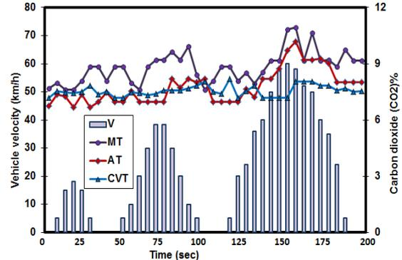
Fig. 14: CO<sub>2</sub> emissions for MT, AT and CVT
