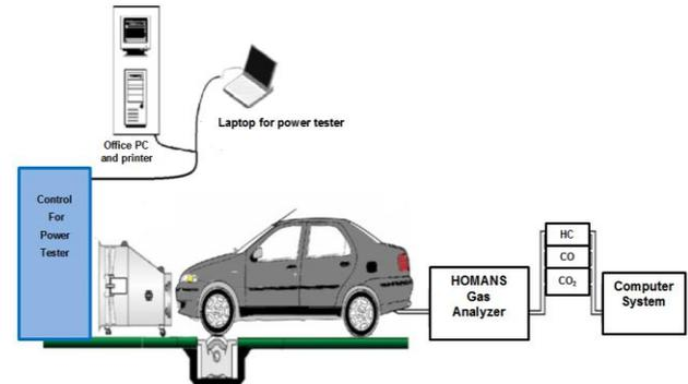
Fig. 3: Schematic of test setup and instrumentation system
